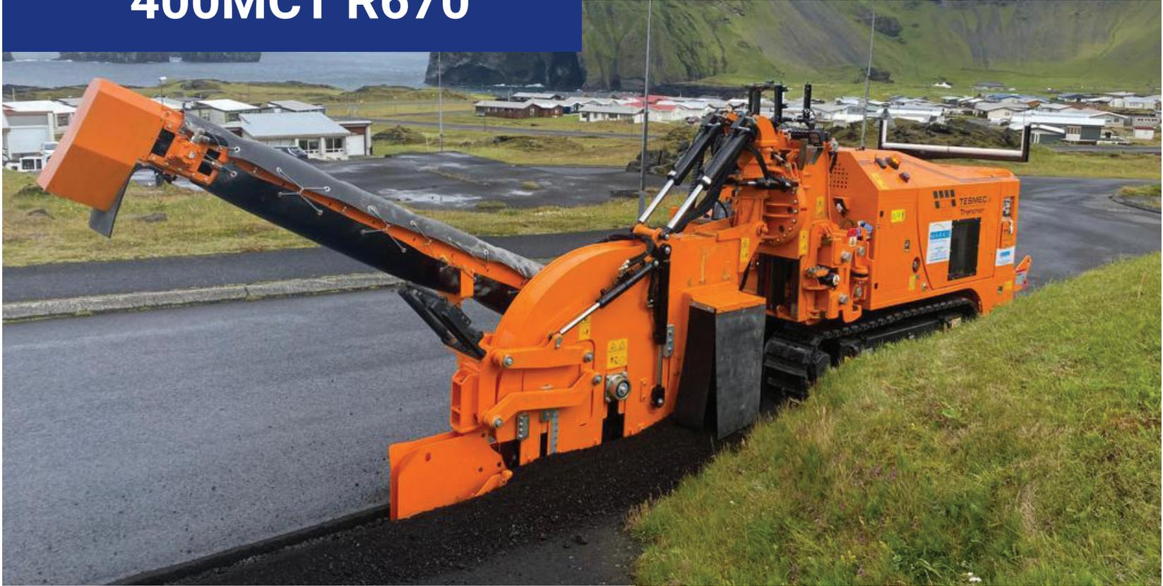
Tesmec 400MCT with R670 is a 11 metric ton-class trencher featuring a 238 Hp (175kW) tier 4/Stage V engine, or a 218 Hp (218 kW) tier 3 engine, designed for telecom and fiber optic projects in urban areas
